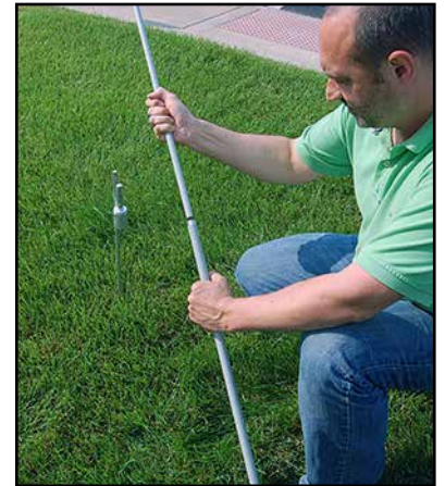
Assemble mast poles. Thickest section into thinnest.
