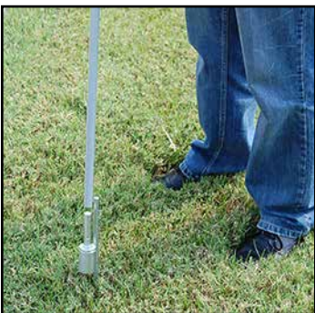
Slide mast bottom onto top of stake.
